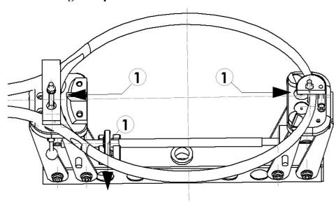
The racquet support is adjusted to the seize of the racquet with the knurled knob on the screw spindle. Put the racquet on the mounting system and place both clamps above the racquet.
