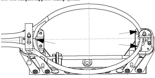
The racquet is supported with 2 supports at the head side and the V-shaped "Babolat retainer" at the
