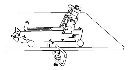
The machine can only be used when it is clamped to the table. Slide the table clamp through the frame and position the machine so far from the edge of the table that the clamping screw is under the centre of the frame. Tighten the clamping screw firmly.
