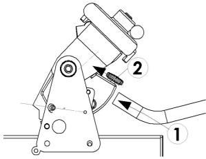
Loosen the clamping screw a little and slide the lever into the tension head with the screw in the slot. Tighten the clamping screw.
