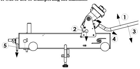
When the machine is out of use or should be transported the tension head should be in the end position against the stop:
