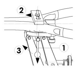
The racquet can be removed by using the slot hole in the cross bar and lift it off the machine. Or by rotating the clamping bar and move it through the open handle of the racquet.
