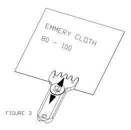
To clamp the string with a minimum clamping force the clamping surface must be equally rough.
