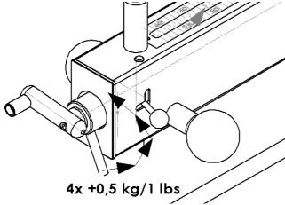
On the MS140L the tension can be raised or lowered in 4 steps of 0,5 kg (1 lbs) with the handle behind the adjusting handle.
