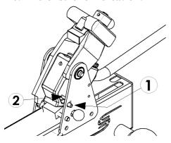
At the end of the stroke the tension drops and the "End of stroke indicationd" moves out. Repull the string without moving the clamp.
