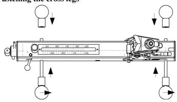
Put the cross leg screws through the frame and the second bush and tighten the ball knob firmly.
