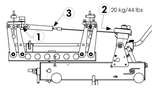
The tension system can be calibrated with the calibrator which is supplied with the machine. The tension will not vary more than a few percent over the hole stroke. To get the most accurate results calibrate the system in the middle of the stroke between the forward position and the moment that the "end of stroke signal" starts to move.
