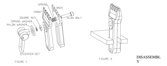
For the disassembly and assembly it is easy to use a vise or a special piece of wood with a slot in it to hold the clamp as shown in figure 2.
