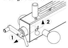
The MS140L has a table lock which locks the turntable in 6 positions. When the lever is in the upper position the table will lock as soon as the locking pin meets a hole in the turntable.
