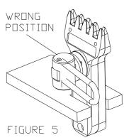
For easy up and down sliding of the clamp it is advised to insert a thick layer of grease into the hollow that clamps the clamp on the pin of the sliding system.
