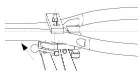
The racquet is clamped with a transparent crossbar so that there is good view on the grommet holes in the bridge of the racquet.
