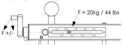
\* The tension can be adjusted between 18 and 28 kg or 32 and 62 lbs. The machine can string up to 32 kg or 72 lbs by adding the extra (badminton) weight.
