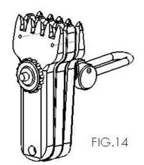
A flying clamps holds the tension by clamping the last string to the string before last.
